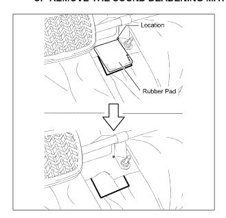
1. Temporarily place the rubber pad on the floor panel as shown, and outline the pad on the sound deadening material with a ball point pen.
